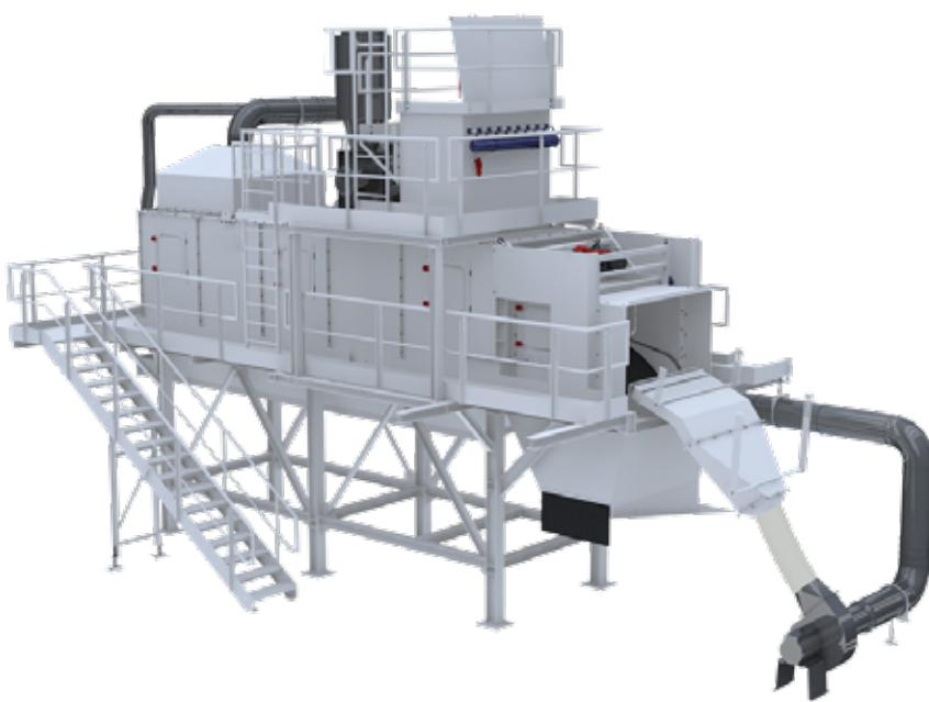
The Windsifter is a rugged equipment with great capacity to separate the light material from the heavy one. The aim of which is the separation of the inert material (stones, scrap, stainless steel) so availability and durability of the secondary shredders of alternative fuels production lines can be increased, thereby assuring a low operating cost.
